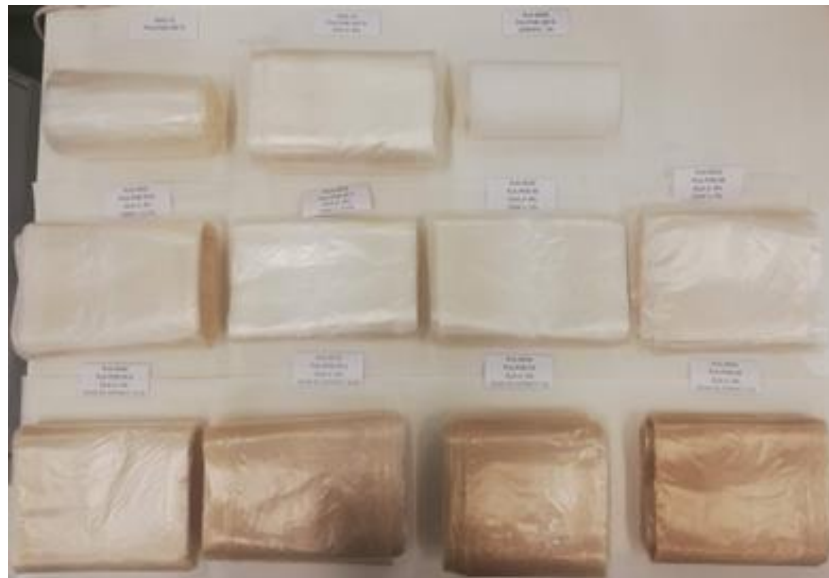
Figure 3: Blown films of the PLA/PHB-based blends produced by Proplast (picture by Tecnopackaging)
