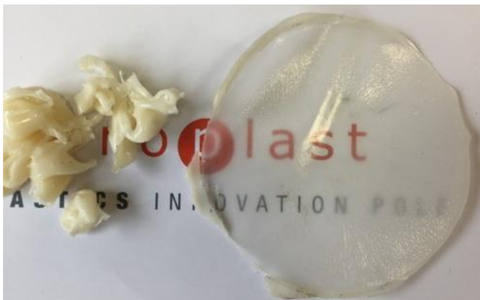
Figure 1: PLA:PHB (60:40) blend with 1 wt.% CNWs and related compression moulded sample
